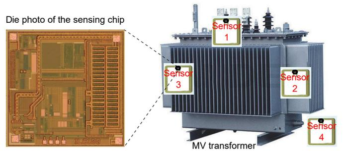
Fig. 1. System block diagram showing the deployment of the sensors (sensor 1: top surface, sensor 2: left radiator, sensor 3: right radiator, sensor 4: hang in the air).
