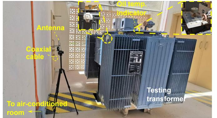
Fig. 3. Test setup with antenna mounted on a tripod and facing transformer and lattice wall
