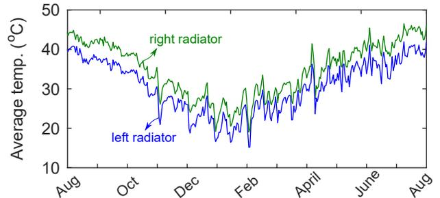
Fig. 7. Temperature profiles of the right and left radiator of the transformer.
