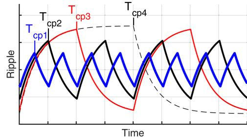
Fig. 2. Comparison of the ripple shapes of four different half chopping periods ( $T_{cp1} < T_{cp2} < T_{cp3} < T_{cp4}$ ).
