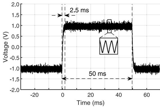
Fig. 6. Step response of the CCIA with a 10 mV input at 20 Hz.
