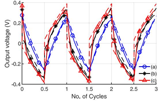
Fig. 8. Chip results (symbols) vs. MATLAB model (dotted lines) of different Miller compensation resistances and second stage transconductances (a)  $R_m = 1/g_{m2}$ , (b)  $R_m > 1/g_{m2}$ , and (c)  $R_m \gg 1/g_{m2}$ .
