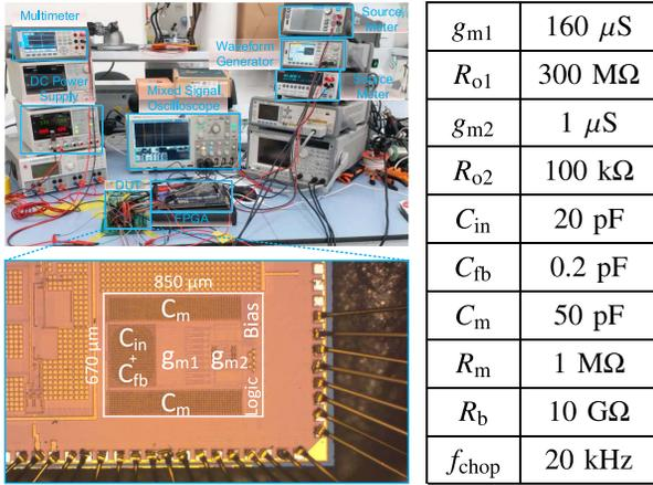
Fig. 5. Experimental setup for verifying the derived analytical model for ripple shapes/amplitudes and design parameters of the prototype chopper amplifier.
