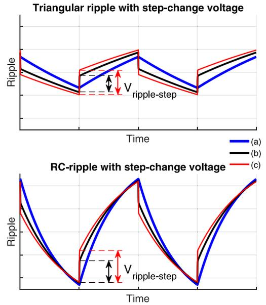
Fig. 4. Effect of the voltage step on triangular ripple and RC-ripple when (a)  $R_m = 1/g_{m2}$ , (b)  $R_m > 1/g_{m2}$ , and (c)  $R_m \gg 1/g_{m2}$ .
