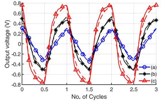
Fig. 7. Chip results (symbols) vs. MATLAB model (dotted lines) of different time constants and half chopping periods (a)  $\tau_{1A} \gg 1/2 \cdot f_{chop}$ , (b)  $\tau_{1A} \approx 1/2 \cdot f_{chop}$ , and (c)  $\tau_{1A} \ll 1/2 \cdot f_{chop}$ .
