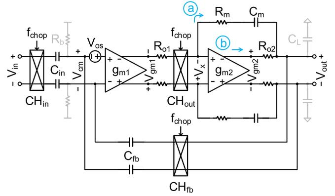
Fig. 3. Illustration of the two signal paths of the second-stage amplifier with nulling resistor (a) the compensation path via  $R_m$  and  $C_m$ , and (b) the forward path via the second-stage output impedance.
