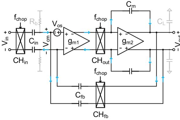
Fig. 1. A typical chopper-based instrumentation amplifier.
